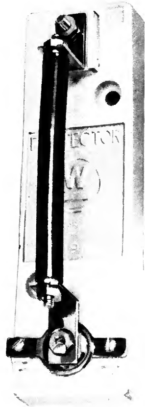
Fig. 6. A popular type of lightning arrester fitted with a fuse to protect the antenna in the event of its coming in contact with high voltage power lines
